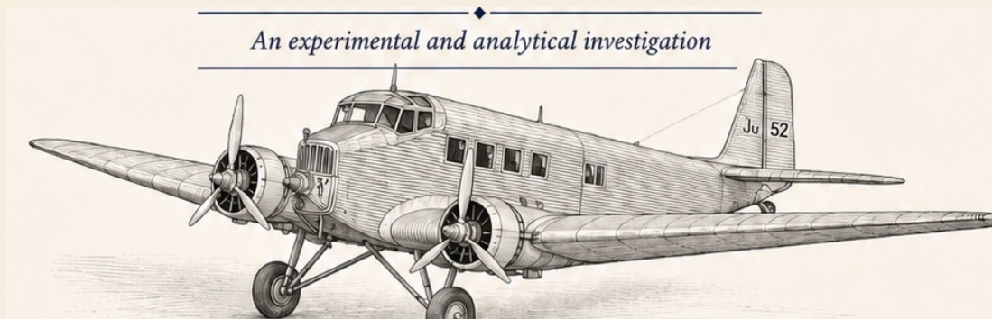
Figure 1.1 - The Ju 52/3m: corrugated external skin, fixed undercarriage, three radial engines and offset trailing-edge surfaces made aerodynamic cleanliness only one of several competing design priorities.
