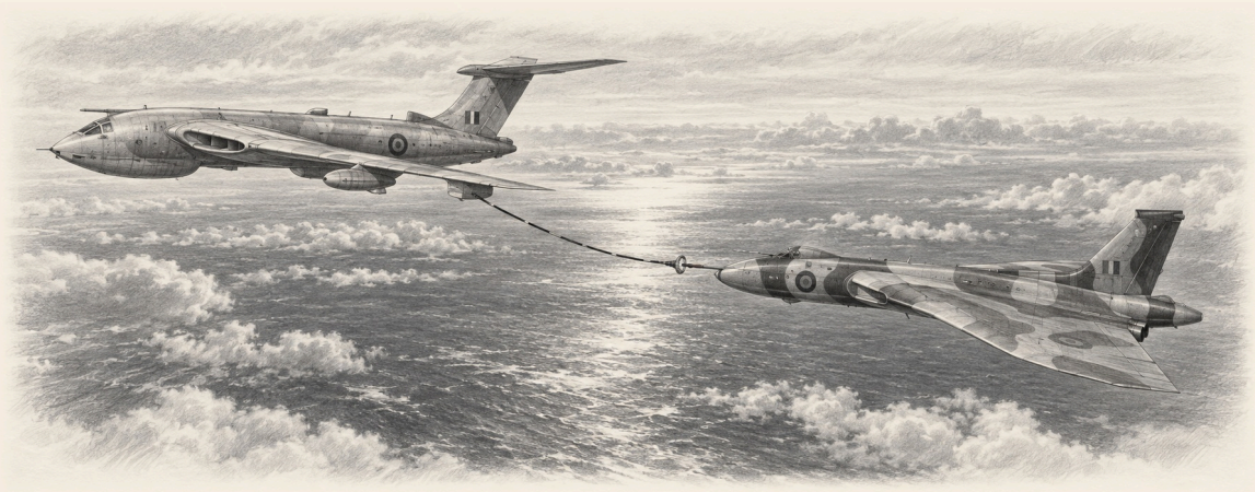
Figure 2.1 - A Vulcan taking fuel from a Victor tanker over the South Atlantic, 1982, the hose and basket clearly shown. The Department wishes the contrast with Chapter 4 to be visible.
